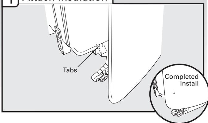
Using the precut slots in the insulation, fasten the insulation over the molded hooks on the tub. Be sure to fasten the insulation down on both sides of the tub.
